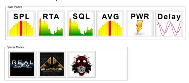
"SPL" - is the mode used for measuring the peak value of the sound pressure level for signals with frequency ranging from 10 to 20 Hz with resolution of 1 Hz. In this mode, the waveform, spectrum and level of the measured signal are reflected. It is possible to measure up to 4 channels simultaneously. In this mode, it is possible to measure the voltage-current characteristics and the sound pressure simultaneously when using appropriate equipment.
